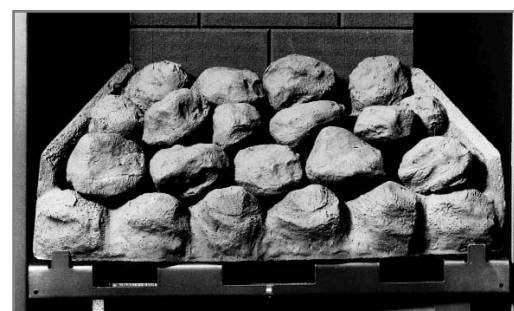
Place the middle row of four coals onto the supports in the matrix, over the top of the holes. Ensure the coals are not turned sideways, such that they actually enter the holes.
