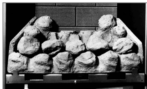
Place the middle row of four coals onto the supports in the matrix, over the top of the holes. Ensure the coals are not turned sideways, such that they actually enter the holes.
